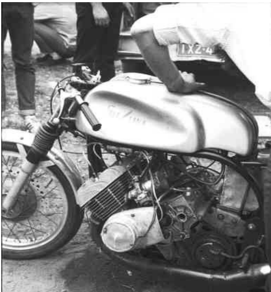
Next Tauno Nurmi bought two Suzuki 250 cm engines and added them together.
