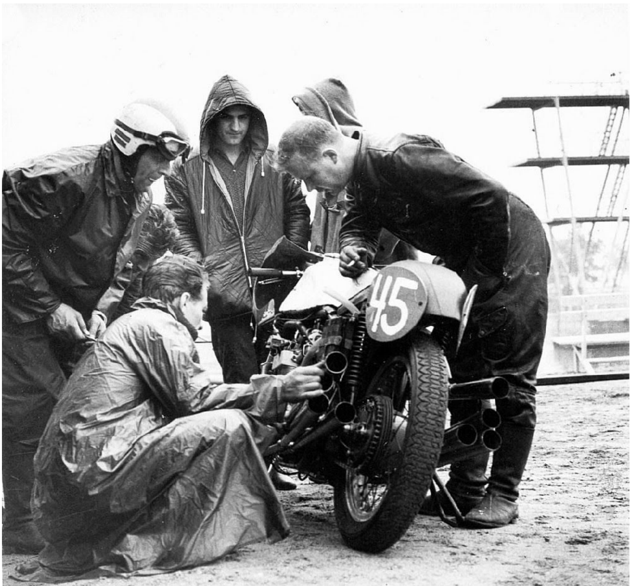
About 1964, Finnish TT motorcyclist technician area lecturer Tauno Nurmi built a 350 cc DOHC V8-powered 4-stroke motorcycle engine by the name V8 PREMIER. V angle is 90° and it is air-cooled. Each cylinder has its own carburettor. It is his own design and construction. You can see the picture from Imatra 1965 and Tauno Nurmi is in left with helmet. Kuva ja lähde: Retro Rog, Imatranajot 1965 ( http://www.imatranajot...urmiV8_1965.jpg ).
