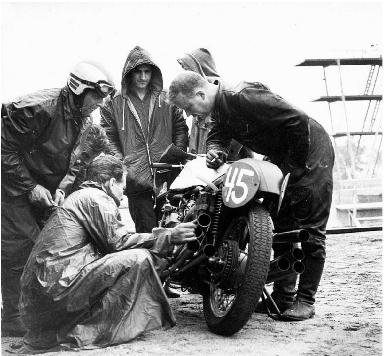
About 1964, Finnish TT motorcyclist technician area lecturer Tauno Nurmi built a 350 cc DOHC V8-powered 4-stroke motorcycle engine by the name V8 PREMIER. V angle is 90° and it is air-cooled. Each cylinder has its own carburettor. It is his own design and construction. You can see the picture from Imatra 1965 and Tauno Nurmi is in left with helmet. Kuva ja lähde: Retro Rog, Imatranajot 1965 ( http://www.imatranajot...urmiV8_1965.jpg ).
